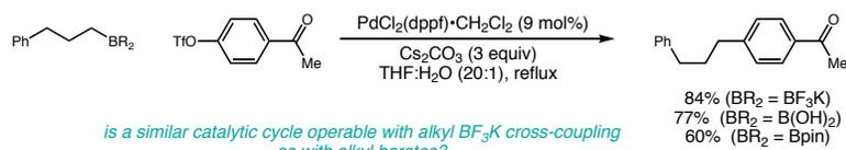
is a similar catalytic cycle operable with alkyl BF<sub>3</sub>K cross-coupling as with alkyl borates?
