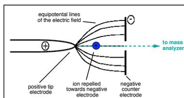
**FD** : the sample is placed directly onto the surface (dipping emitter in an analyte solution) before ionization but FD is needed for non-volatile and/or thermally labile substances.
