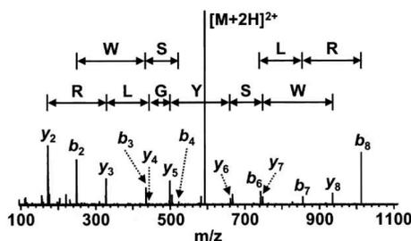
SORI-CID fragment ion spectrum of human luteinizing hormone-releasing hormone using 7 Tesla FT-ICR MS. All amide bonds, except the two closest to the *N*- and *C*-termini, were cleaved in this 10-residue peptide, resulting in a sequence tag of six amino acid residues from the *y* ion series
